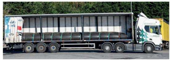
number of our standard curtain-sided trailers are fitted with a 18,000-litre collapsible neoprene tube designed to safely hold liquid-based resin. This product is used as a bonding agent in the manufacture of panelboard. On the return journey from the production site, the trailers have plenty of room to carry finished boards.
