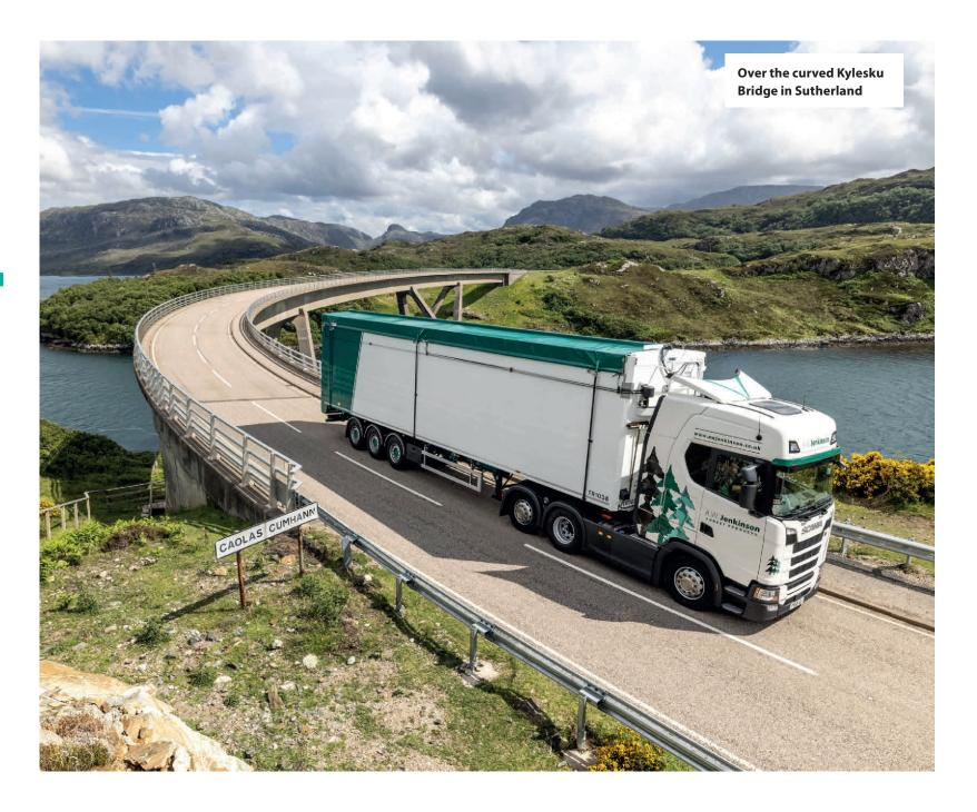
alking floors and chipliners are designed to transport dry bulk products – usually wood chips, wood fibres or recycled wood products.
