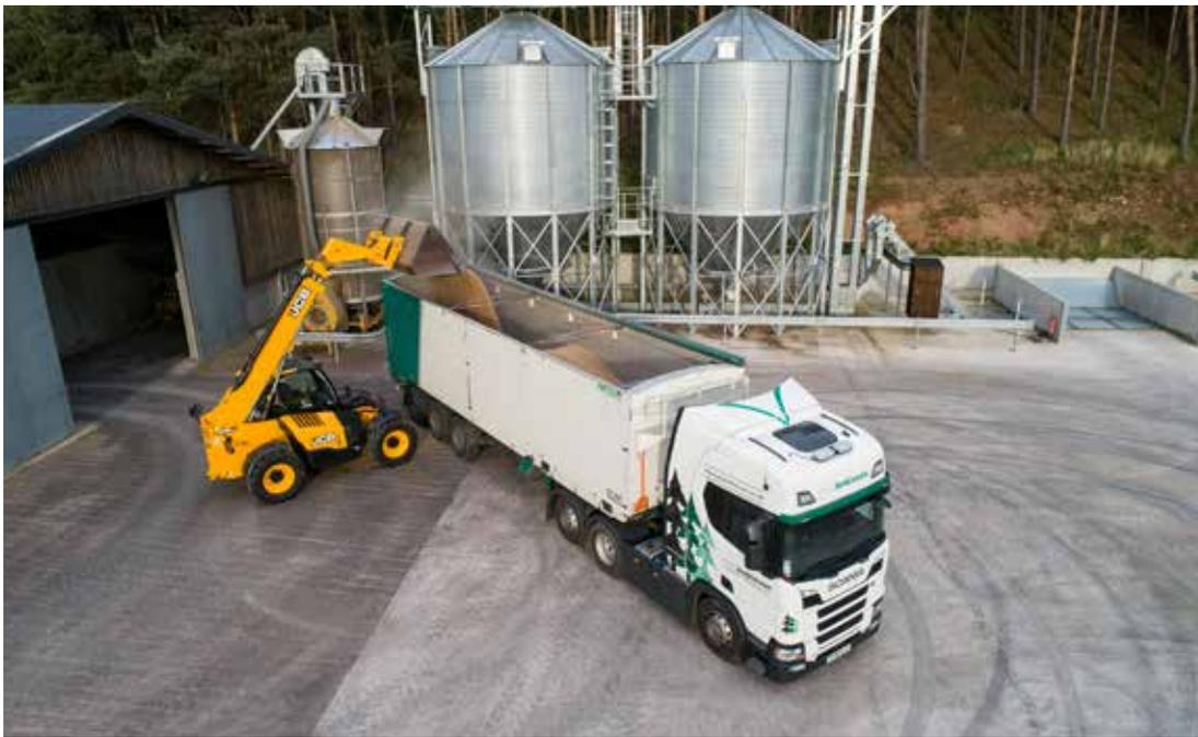
Tipper trucks were the first vehicles used by A.W. Jenkinson more than five decades ago and they remain an important part of the fleet. These roof-loaded, open-topped vehicles are mainly used for transporting bulk materials such as wood co-products to sites with restricted access. They use hydraulic rams to tip their loads out of the rear gate.
