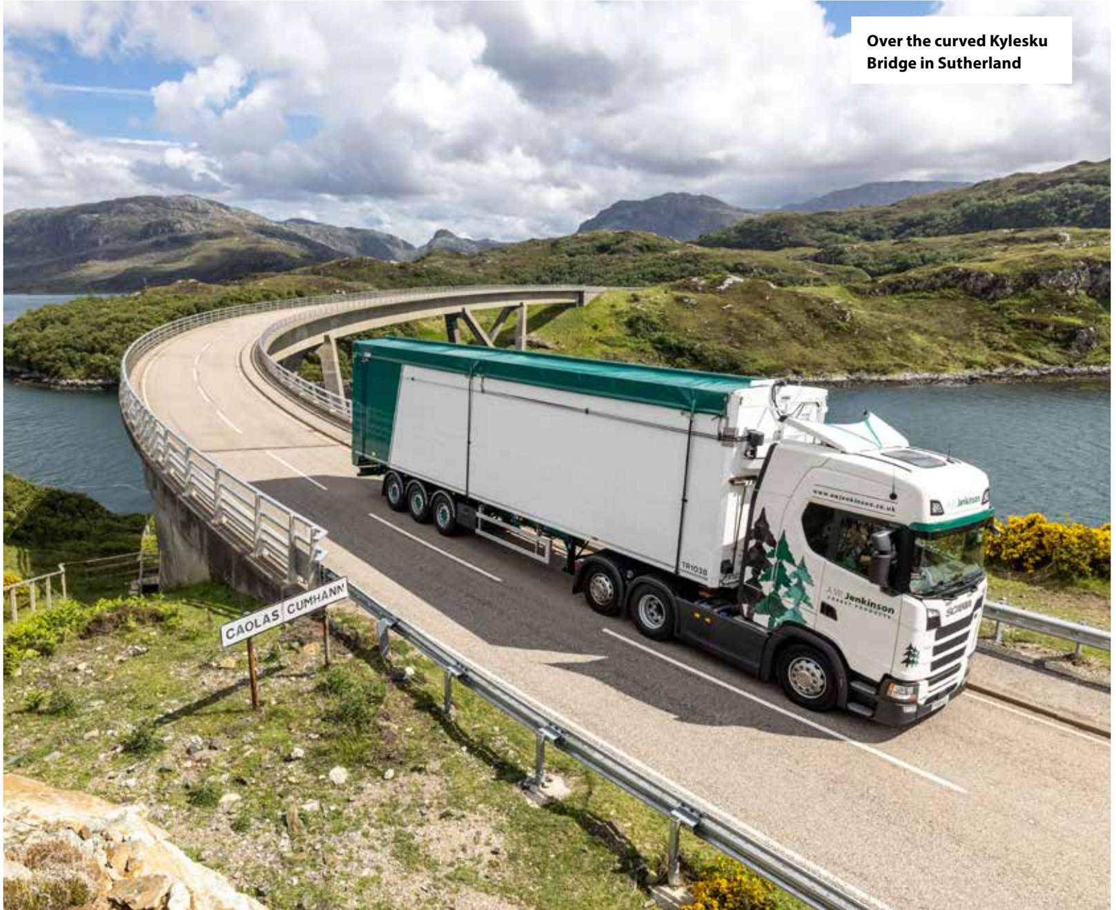
**W**alking floors and chipliners are designed to transport dry bulk products – usually wood chips, wood fibres or recycled wood products.
