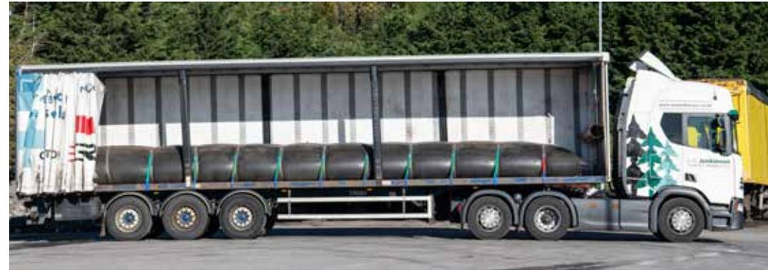
**A** number of our standard curtain-sided trailers are fitted with a 18,000-litre collapsible neoprene tube designed to safely hold liquid-based resin. This product is used as a bonding agent in the manufacture of panelboard. On the return journey from the production site, the trailers have plenty of room to carry finished boards.
